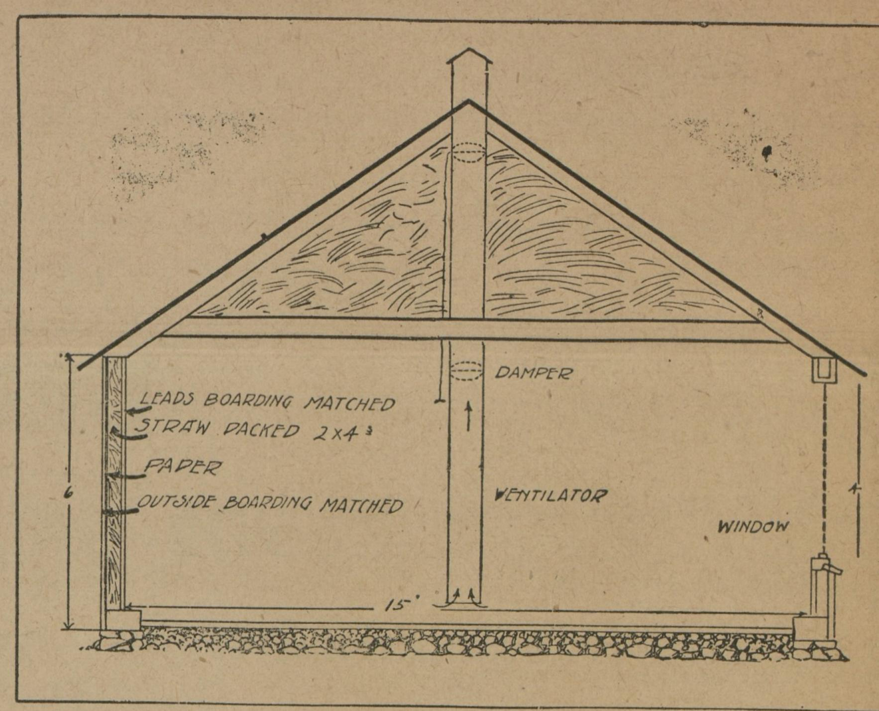
In the colder months when the inside temperature is higher than that outside, the renewal of air can be effected by a central shaft leading up
